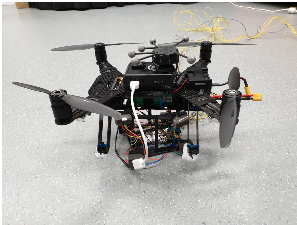
Fig. 5. Side-view of the drone/array set-up. The white cable is the Micro-B USB 3.0 OTG cable and connects the drone's power supply to a PCB, pictured at the bottom of the array, which serves as the power rails for the microphones
