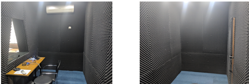
Figure 4: Inside of the acoustic anechoic chamber used for our data collection.
