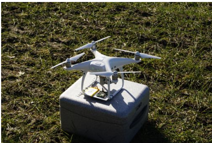
Figure 1: Recording setup consisting of the DJI Phantom 4 PRO Professional Drone and the recording board with battery power supply. The microphone array is fixed on the bottom side.
