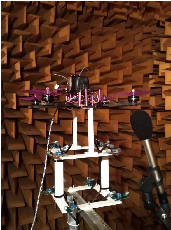
Fig. 2: Microphone array attached to the drone and additional Microphone
