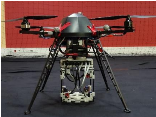
Figure 1. Setup used for the SPCup2019: A Mikrokopter UAV equipped with an array of 8 microphones
